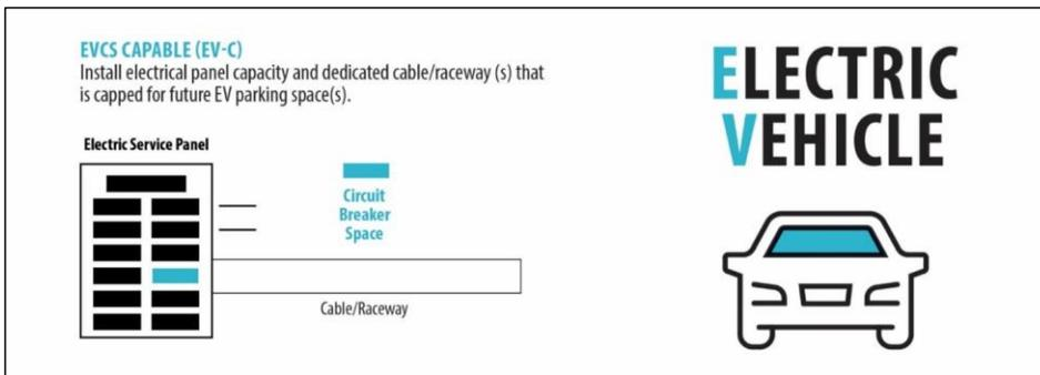
dedicated branch circuit(s) including conductor in a raceway or direct buried, terminated in an approved method in a junction box, for an EV Parking Space(s) (See [Figure 0-2](#)/[Figure 19-2](#)). The junction box shall be clearly marked and labeled with the following text: EV Ready Circuit.
