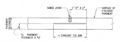
+ EPOXY COATED #5 DEFORMED BAR 2'-6" LONG FOR SYMBOL (D) EPOXY COATED #5 SMOOTH BAR 2'-6" LONG FOR SYMBOL (S) (MAXIMUM ALLOWABLE LANE TIE SPACING SPECIFIED BELOW)
