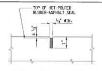
SAWED JOINT SEALED WITH HOT - POURED RUBBER - ASPHALT
