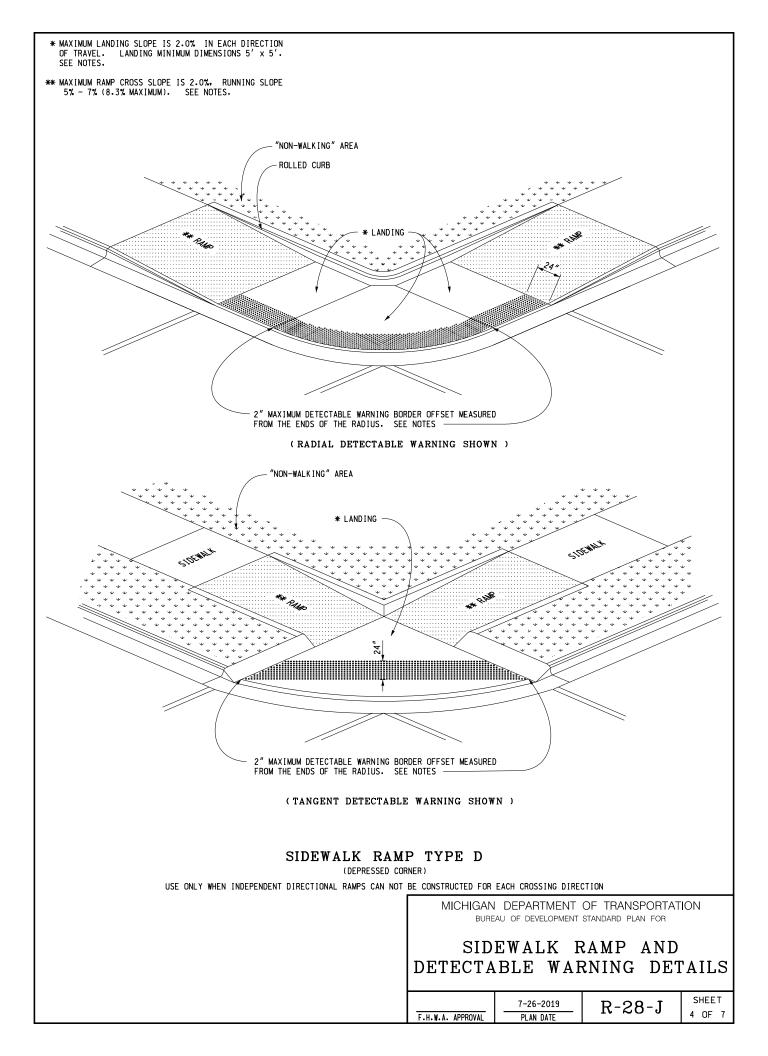
\* THE DETECTABLE WARNING SURFACE SHALL BE LOCATED SO THAT THE EDGE NEAREST THE RAIL CROSSING IS 6' MINIMUM AND 15' MAXIMUM FROM THE CENTERLINE OF THE NEAREST RAIL. DO NOT PLACE DETECTABLE WARNING ON RAILROAD CROSSING MATERIAL.
