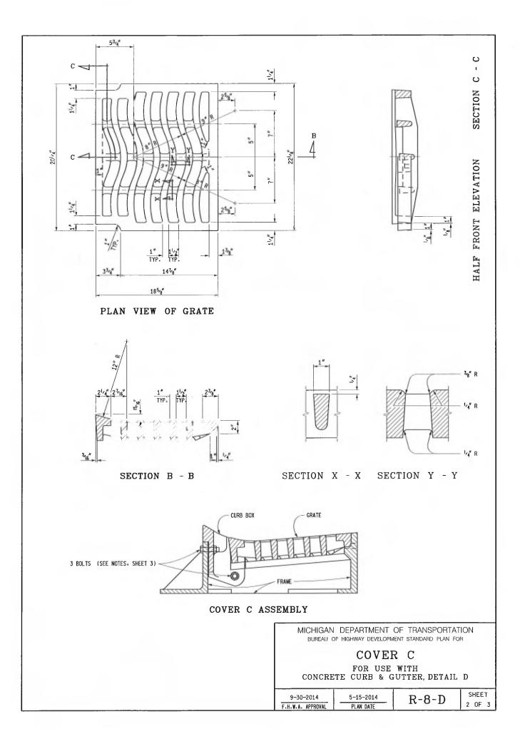
NOTE: BOLT CURB BOX FIRMLY TO FRAME AT FOUNDRY WITH THREE 5g DIAMETER x 21g GALVANIZED MACHINE BOLTS WITH WASHERS AND NUT ENDS. (SEE NOTES)
