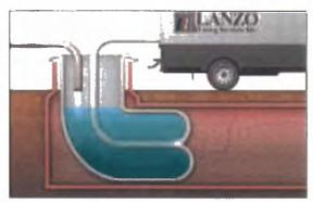
figure1: Direct inversion installation per ASTM F1216
