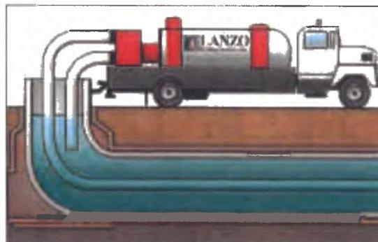
figure 4: Curing liner with hot water or steam
