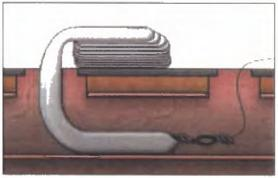
figure 2: Liner pulled-in-place per ASTM F1743
