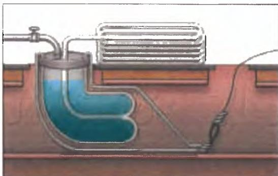
figure 3: Calibration hose or pre liner utilization
