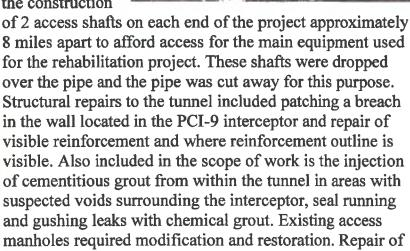
localized cracks and fractures using chemical grout, interceptor lining of selected locations and CCTV inspection after completion of repairs.
