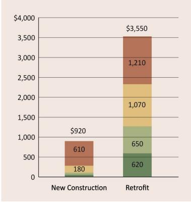
The case study considers a parking lot with ten total spaces and two EV parking spaces, and compares the EV infrastructure installation costs at the time of new construction versus building retrofit. "EV parking spaces" define spaces that have an EV-ready outlet, and include the electrical panel capacity, raceways, breakers, outlet boxes, and wiring to install an EV charger at any given time in the future.
