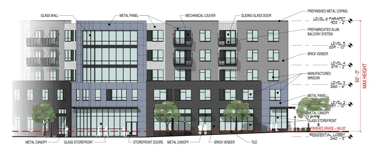
2 PACKARD ST. ELEVATION SP-10 SCALE: 1/16" = 1'-0"
