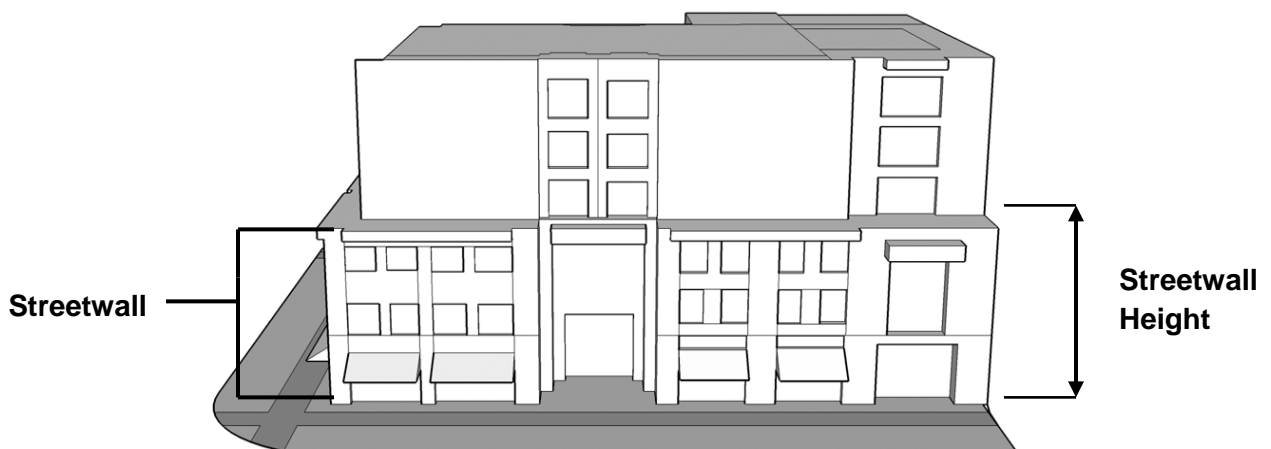
Figure 7: Streetwall and Streetwall Height
