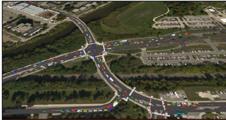
WSP recently used VISSIM for an operations analysis of the Fuller/Maiden Lane intersection to capture multi-modal impacts of different design alternatives.
