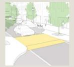
Speed tables are typically 22 feet wide – including a 10 foot wide center platform and slopes tapering down on each side, 3 inches high and extend the full width of the street. The center platform width is variable and can be customized to the location.
