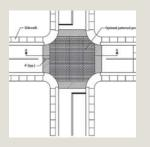
A raised intersection involves ramping each side of an intersection approach and raising the entire intersection 3 inches. Where there are pedestrian crossings, crosswalks can also be marked and raised to the elevation of the raised intersection.
