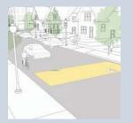
Speed humps are 12 feet wide, 3 inches high, have a parabolic shape, and extend the full width of the street.
