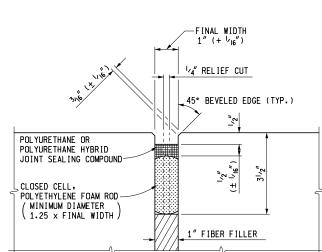
SAWED JOINT DETAIL SAWED JOINT SEALED WITH POLYURETHANE OR POLYURETHANE HYBRID JOINT SEALING COMPOUND. NOTE:
