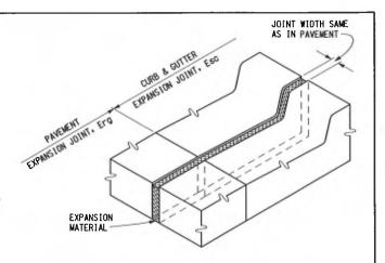
CURB, GUTTER, AND CURB FACE SHALL BE SAWED AS DEEP AS THE EXISTING PAVEMENT THICKNESS. THE REMAINING CONCRETE SHALL BE CHIPPED OUT AND EXPANSION MATERIAL OF SUFFICIENT THICKNESS SHALL BE PLACED IN SAWED JOINT TO FILL THE GAP AS DIRECTED BY THE ENGINEER.
