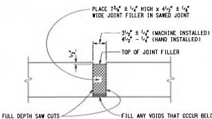
FILL ANY VOIDS THAT OCCUR BELOW FILLER WITH STRIPS OF URETHANE FOAM OR POLYETHYLENE FOAM
