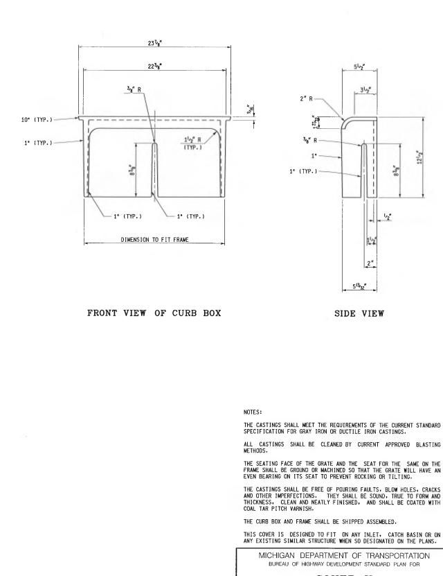
COVER K FOR USE WITH CONCRETE CURB & GUTTER
