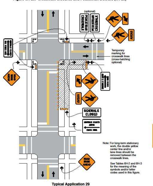
Figure 6H-29. Crosswalk Closures and Pedestrian Detours (TA-29)
