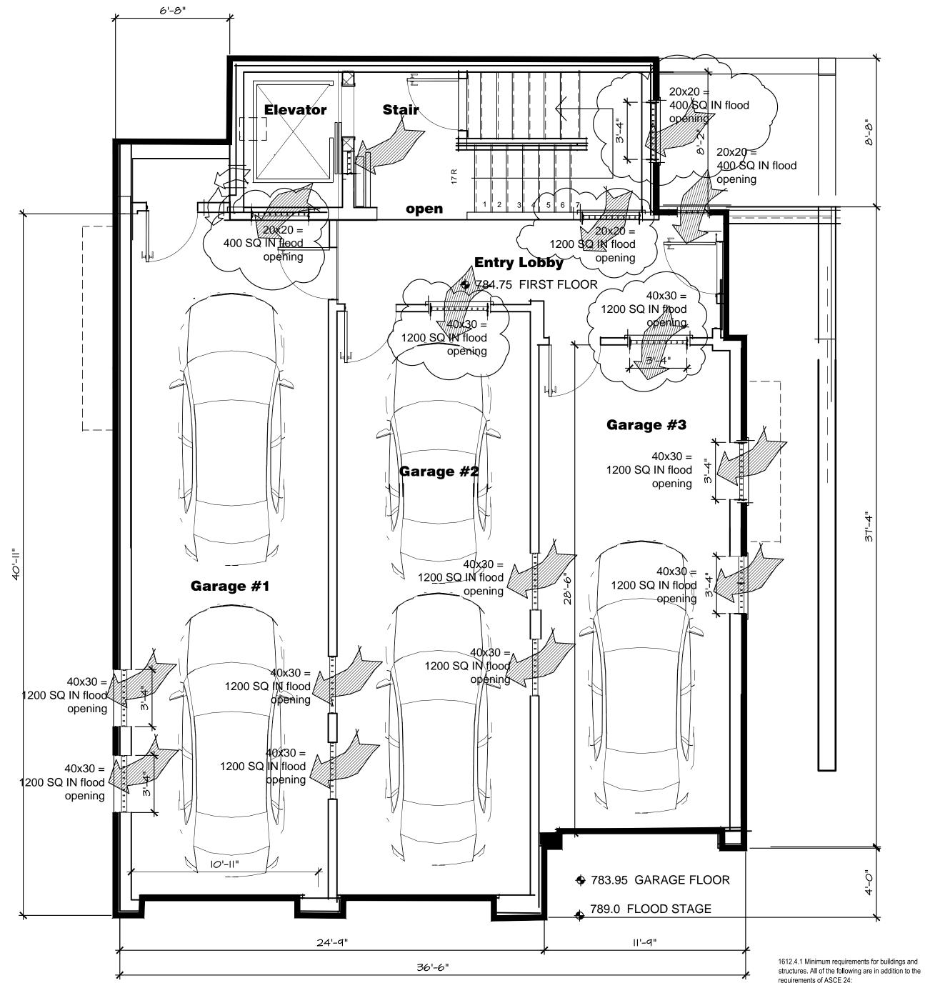
FLOOD EQUALIZTION REQUIREMENTS 1635 SF: FLOOR AREA 1635 Sq In - Flood Window Required 2400 Sq In - Flood Window Provided
