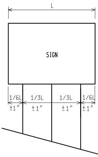
\* FOR ALL 11' AND 12' LONG SIGNS ON 3 WOOD SUPPORTS, SPREAD POSTS SO AS TO HAVE A 8' MIN. TO 9' MAX. DISTANCE BETWEEN OUTSIDE POSTS.
