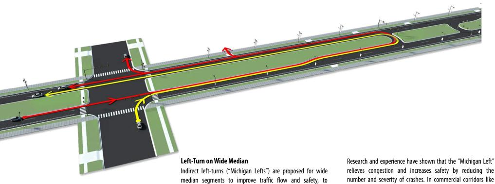
relieves congestion and increases safety by reducing the number and severity of crashes. In commercial corridors like Washtenaw Avenue, crossovers typically need to accommodate a 74-foot overall length truck with a 45-foot turning radius.
