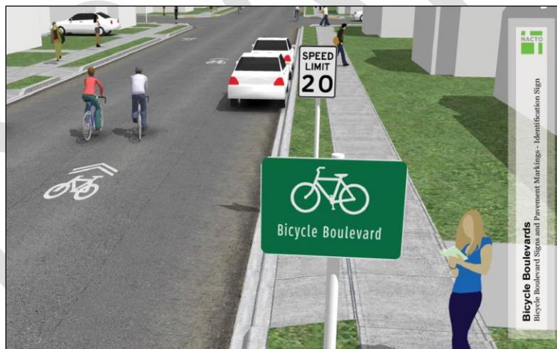
Figure 1 – NACTO Urban Bikeway Design Guide Bicycle Boulevard: Signs and Pavement Markings
