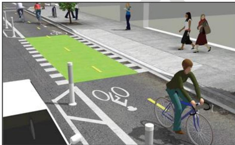
*Figure 2 – NACTO Urban Bikeway Design Guide Two-Way Cycle Track Illustration*
