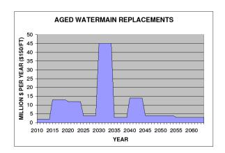
These graphs show that starting in approximately 2016 there is likely to be an increasing need to replace water main pipes within the system. This increase in reinvestment is anticipated to be in the range of 10 times the current rate of replacement. The actual need will be identified as the mains age.
