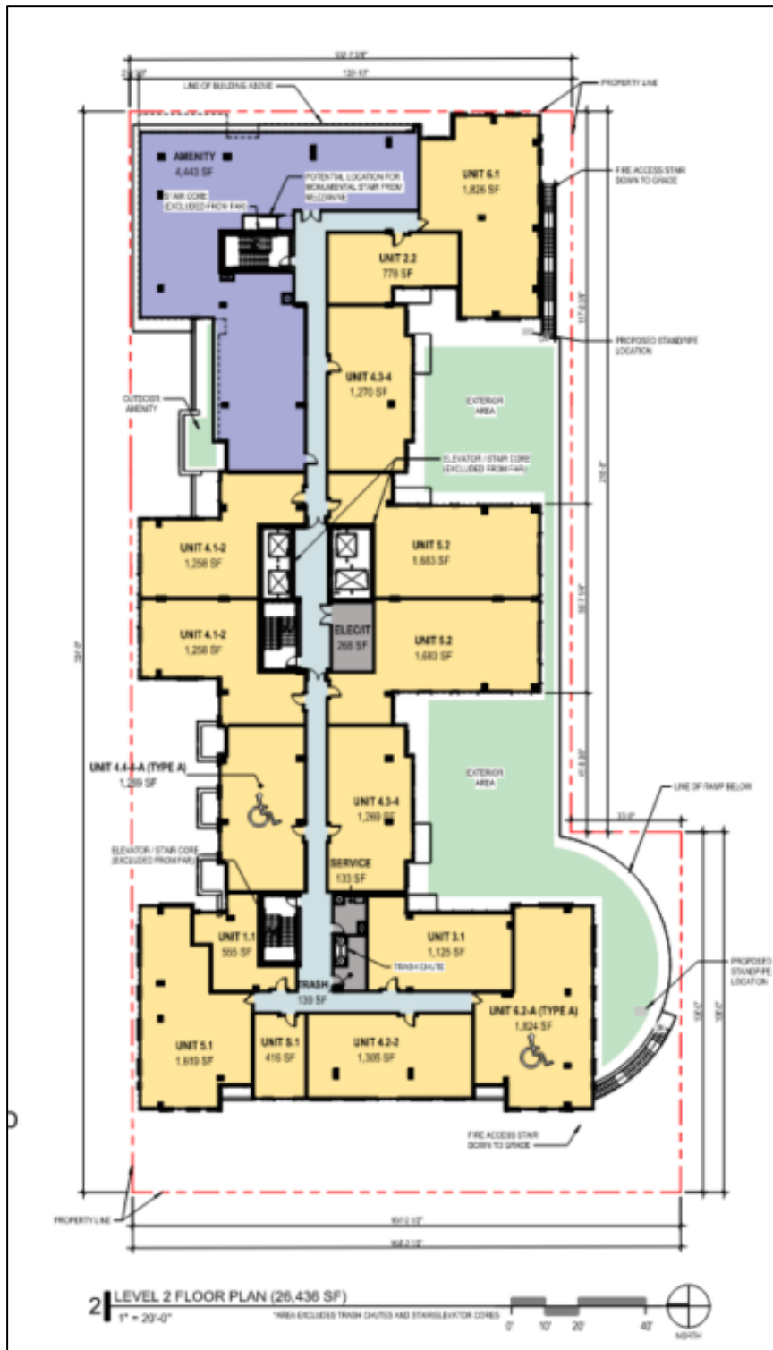
Figure 4: Proposed level 2 floor plan. Base includes green shading (depicting open space on top of base). Tower includes only purple (amenity space) and yellow shading (apartment units). Red dashed line illustrates site boundary.
