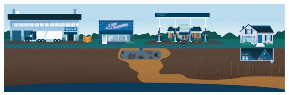
This illustrates a chemical spill from an underground storage tank that entered the ground, moved through the soil and groundwater to an area where vapors from the spill could enter a nearby home.
