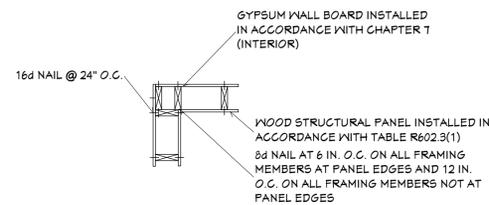
FIGURE R602.10.5 - CORNER FRAMING OUTSIDE CORNER DETAIL
