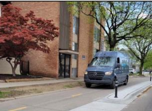
In May, 2022, the DDA and City installed delineators at the beginning and end of key Downtown Bikeway access locations. These yellow posts accommodate standard street sweepers but deter the accidental offender. Most bikeway blocks have loading zones, service alleys, and/or driveways to appropriately accommodate delivery vehicles.
