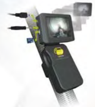
Pole-mounted wireless viewer/recorder stores up to 32 GB of video and images.
