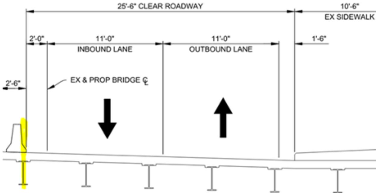
The stage 2 traffic plans detail the installation of temporary concrete barrier wall around the corner of E. Medical Center and W. Medical Center as depicted below. The use of 10-foot barrier wall sections may not be able to create this tight radius, and if not, alternatives will need to be developed.
