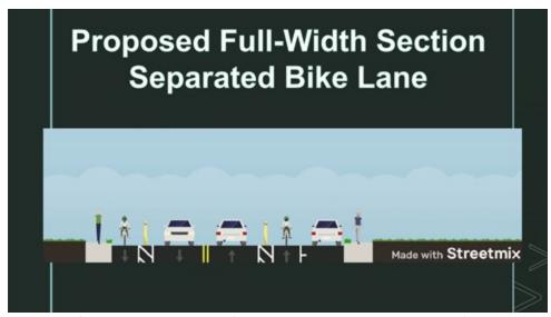
The idea of a separated bike lane (separated by delineators or a curb) is that cars should not cross into that space. Ideally, delineators should be placed closely enough together that cars cannot cross without hitting them. But, in this scenario, putting street parking behind the delineators renders them utterly pointless. The design should be the other way around.
