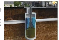
Fig. 2 Maintenance is performed with a vacuum truck.
