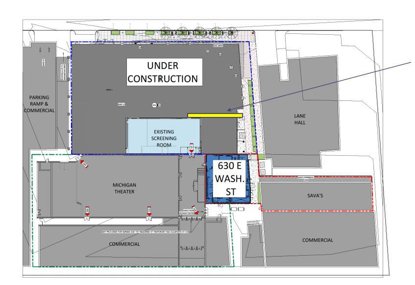
**VARIOUS EGRESS** ROUTES FROM THE NORTH EGRESS DOOR THROUGH THE CONSTRUCTION SITE WILL BE MAINTAINED PER SECTION 3306 PROTECTION OF PEDESTRIANS, ONCE LEVEL 5 FLOOR SLAB HAS **BEEN** COMPLETED.
