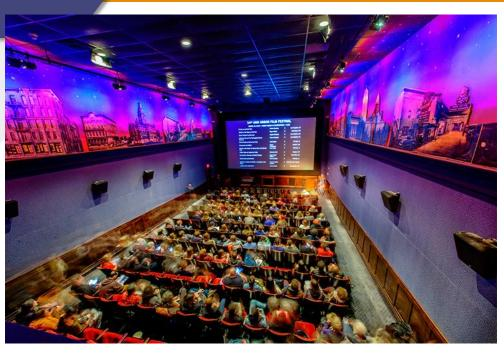
The screening room has occupancy for egress of 257 in it's current configuration based on the original code plans. This occupancy would not be allowed in the Screening Room until 2 means of egress are in place. This would include an exit to the north through 616.
