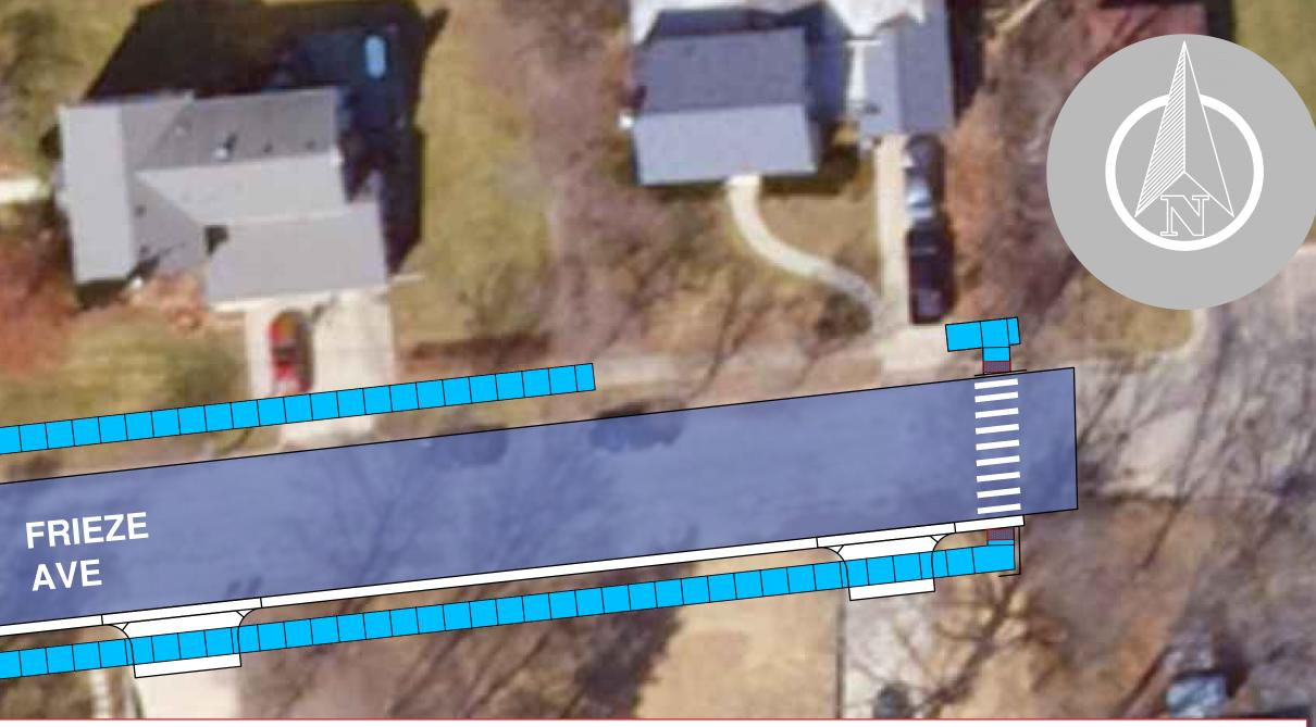
PLANNED AREA OF 12" WATER MAIN CONSTRUCTION IN FRIEZE AVENUE. ALSO, WE PLAN TO FILL THE SIDEWALK GAPS ON BOTH SIDES OF THE ROAD.
