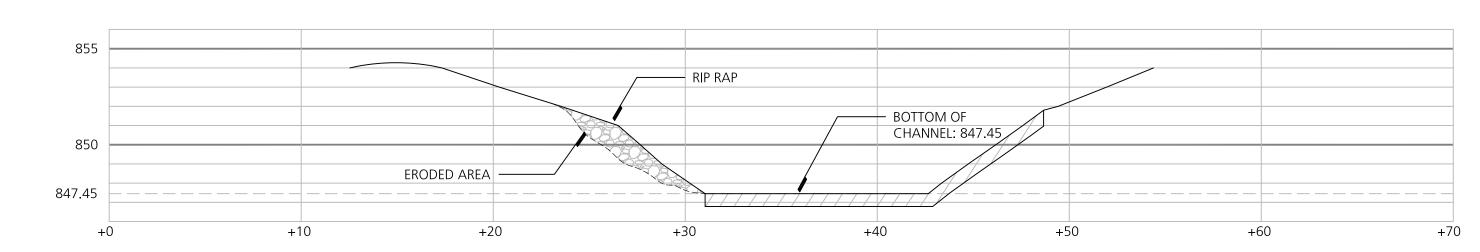
Concrete Channel Cross Section B-B' (Looking West)
