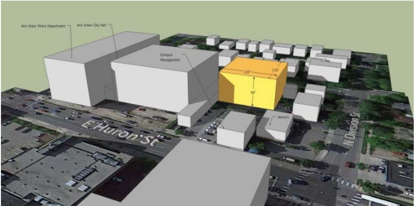
FIGURE 6: THE SITE AS IT COULD BE BUILT OUT UNDER D2 ZONING WITH A 60 FT. HEIGHT MAX.
