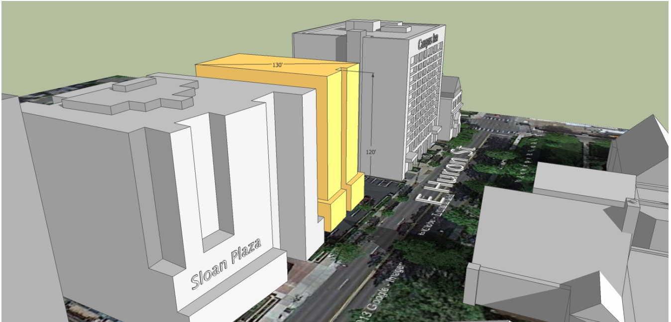
FIGURE 12: EXAMPLE OF A BUILDING CONSTRUCTED UNDER D1 WITH A REDUCED HEIGHT AND A DIAGONAL REQUIREMENT, LOOKING EAST
