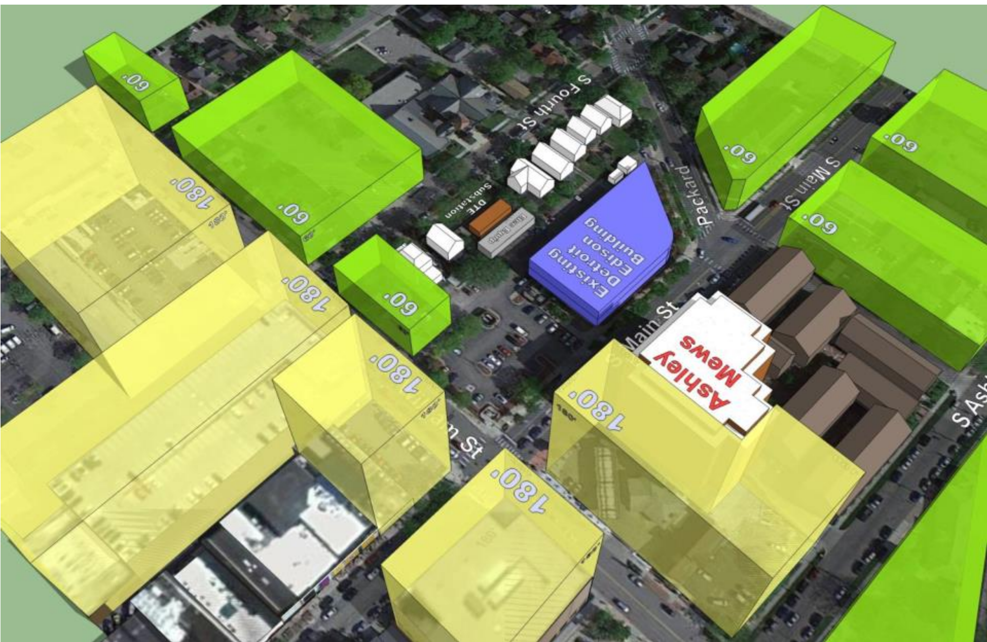
Existing Aerial View looking Southeast showing Allowable Neighboring D1-180' and D2- 60' Heights
