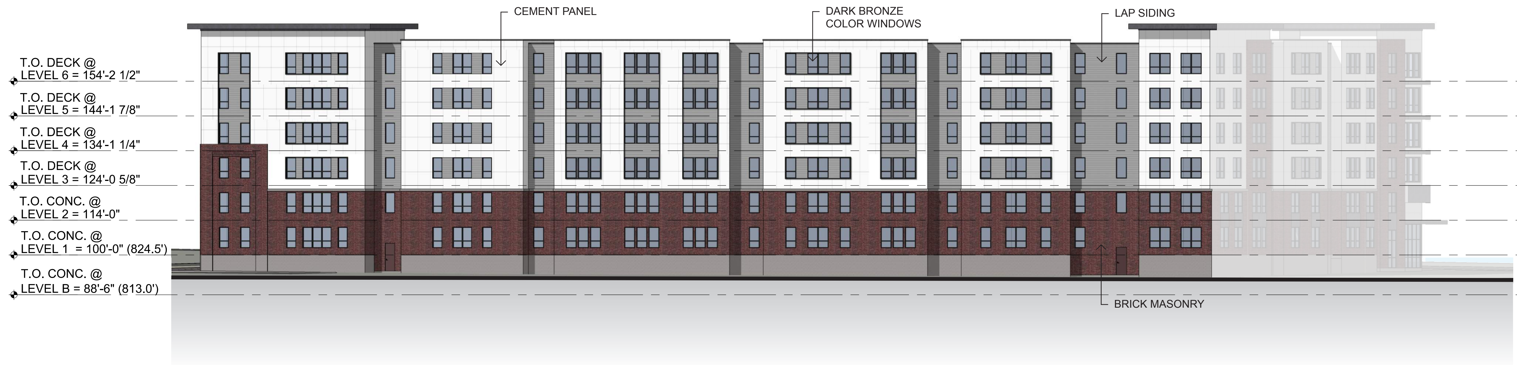
EAST ELEVATION (RAILROAD)
