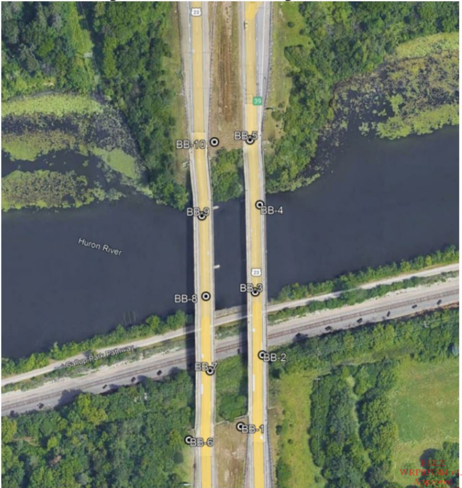
Figure 1. Ro1-1/Ro1-2 Boring Locations
