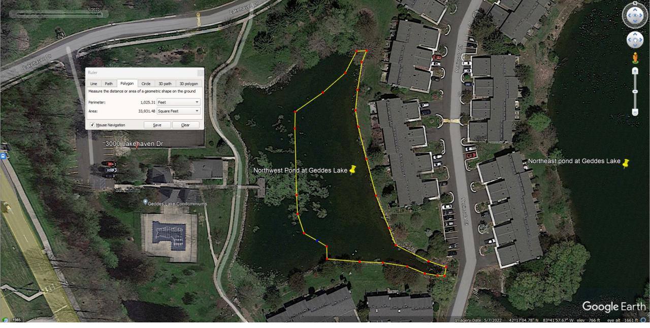
Segment 2, sketch of the sediment removal area for segment 2 in the Northwest pond = 33,931 square feet or 0.77 surface acres.. The removal of an average of 2-feet of organic sediment from this area will result in the removal of approximately 251 cubic yards of dewatered sediment.
