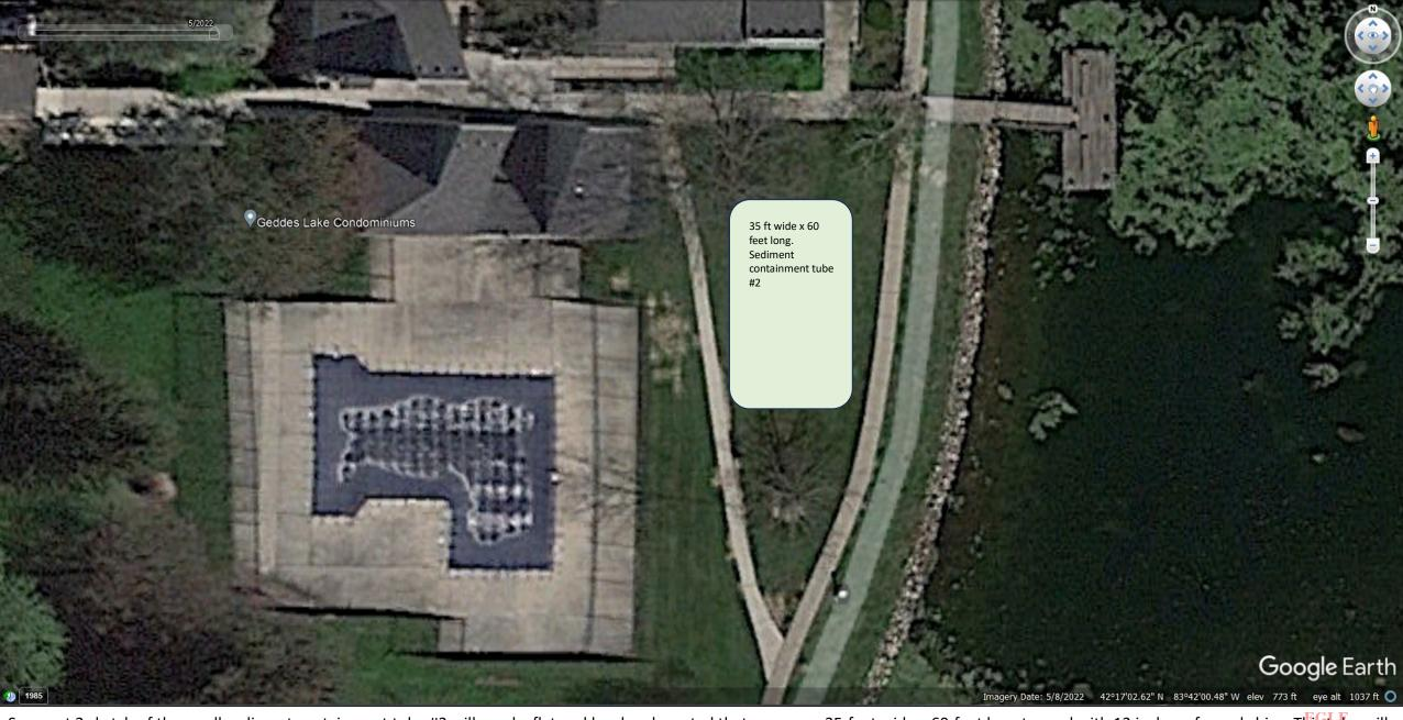
Segment 2 sketch of the small sediment containment tube #2 will need a flat and level pad created that measures 35-feet wide x 60-feet long topped with 12 inches of wood chips. This tube will yield approximately 65 to 70 cubic yards of dewatered sediment. Once filled, the sediment containment tube will need to lay and dewater for up to 10 to 12-weeks until it can be hauled away.
