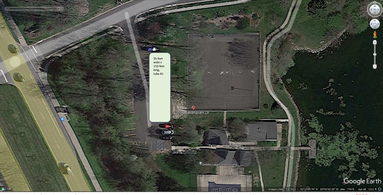
Segment 2 sketch of the placement of sediment containment tube #1. This sediment tube area will measure 35-feet wide x 110-feet long. It will displace several parking spaces however with lot will continue to have limited use. This sediment tube will need to lay and dewater for 10 to 12 weeks or until the sediment is dewatered to the point it can be hauled away. This tube will yield approximately 200 to 220 cubic yards of dewatered sediment.
