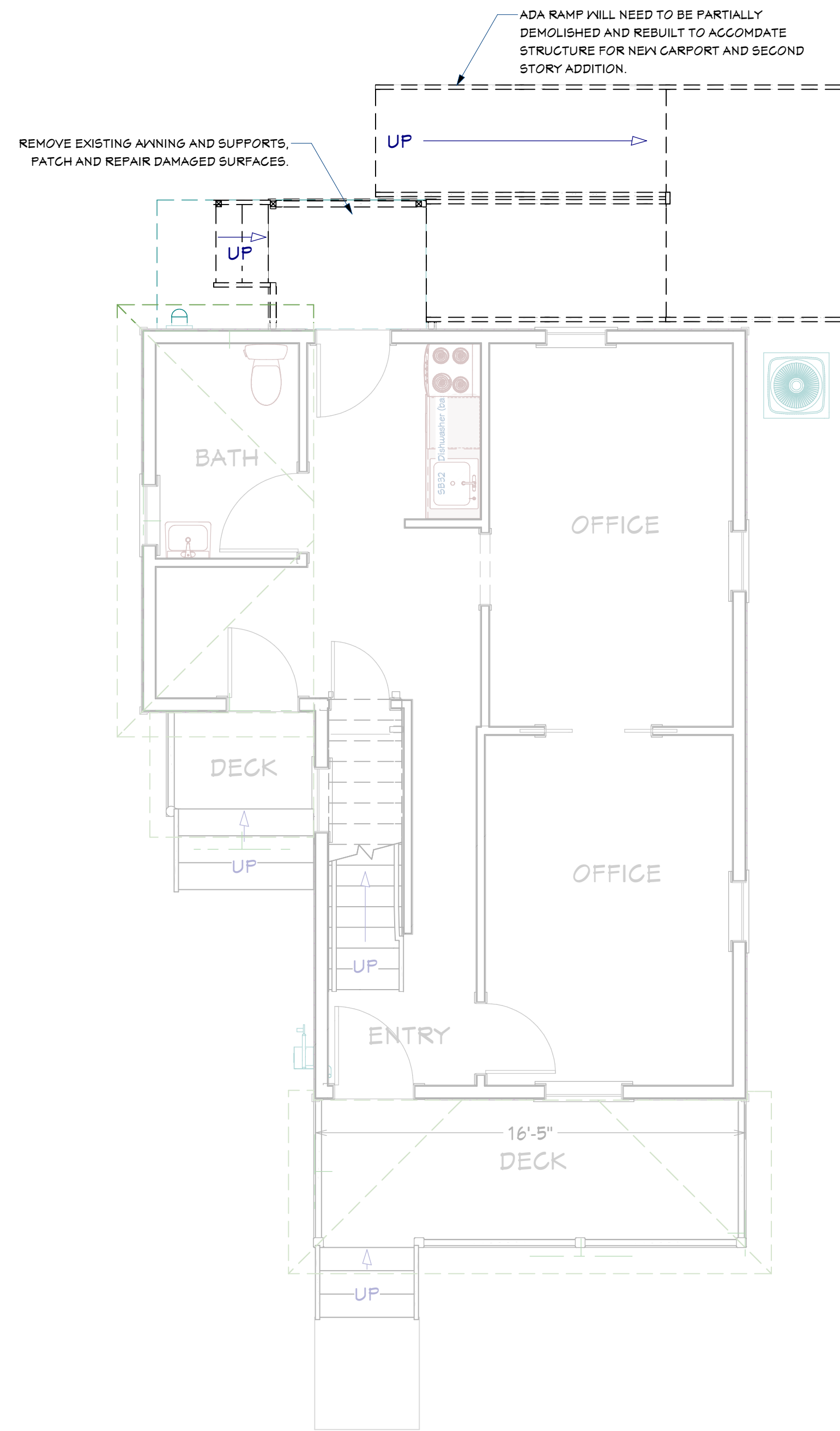
D1 DEMOLITION FIRST FLOOR PLAN SCALE: 1/4"=1'-0"
