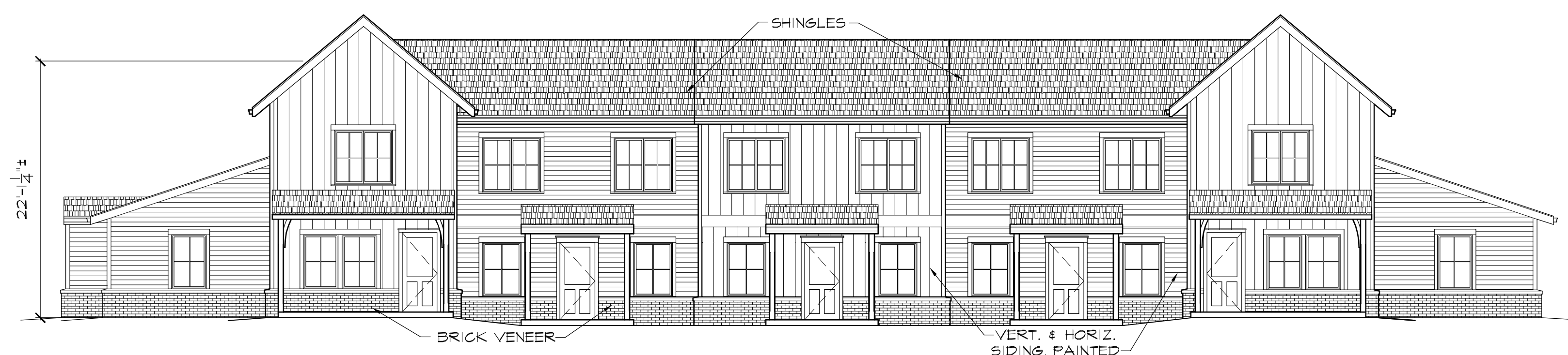
BUILDING I FRONT (NORTH) ELEVATION 1/8" = 1'-0"
