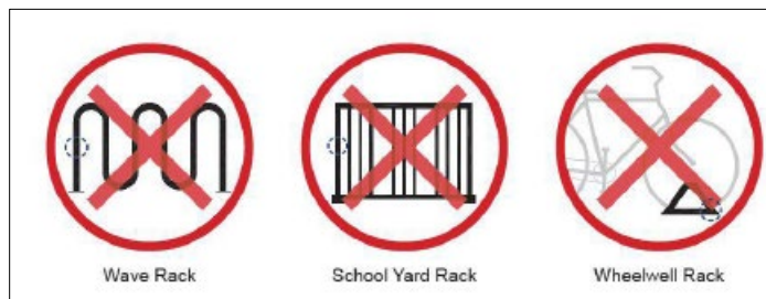
Fig. 19-1: Prohibited Bicycle Parking Racks (source: 2024 AASHTO Guide for the Development of Bicycle Facilities)
