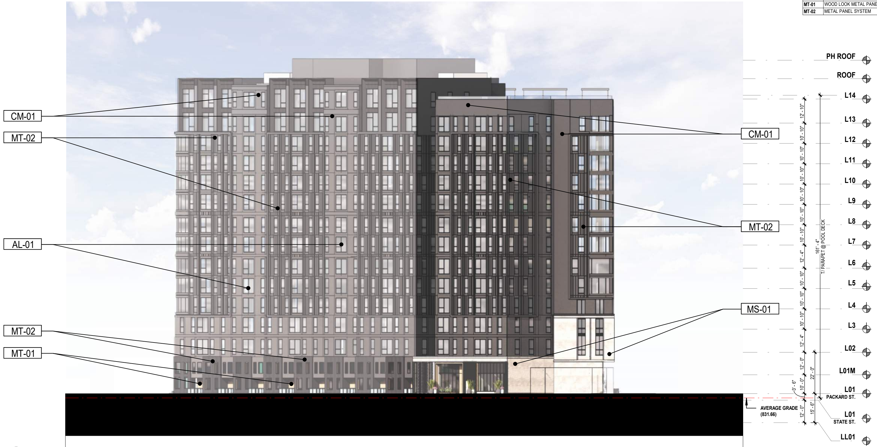
1 EXTERIOR BUILDING ELEVATION - NORTH P3.3 SCALE: 1" = 30'-0"
