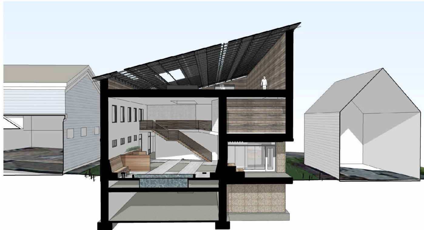
North South Building Section at Entry
