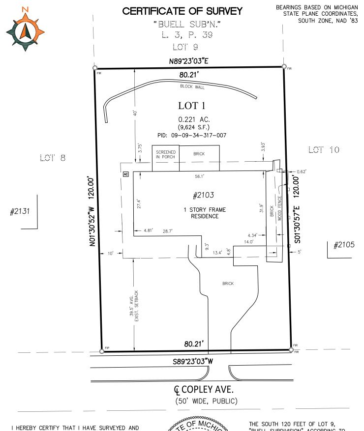
MAPPED THE LAND ABOVE PLATTED AND/OR DESCRIBED ON NOVEMBER 14, 2023, AND THAT THE RATIO OF CLOSURE ON THE UNADJUSTED FIELD OBSERVATIONS OF SUCH SURVEY WAS 1:5000, AND THAT ALL OF THE REQUIREMENTS OF P.A. 132, 1970, AS AMENDED, HAVE BEEN COMPLIED WITH.
