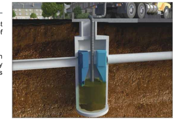
Fig. 2 Maintenance is performed with a vacuum truck.
