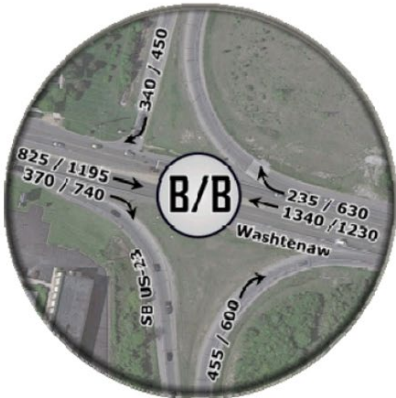
US-23 & Washtenaw (Southbound Ramps)
