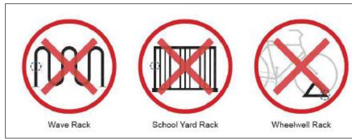
Fig. 19-1: Prohibited Bicycle Parking Racks (source: 2024 AASHTO Guide for the Development of Bicycle Facilities)
