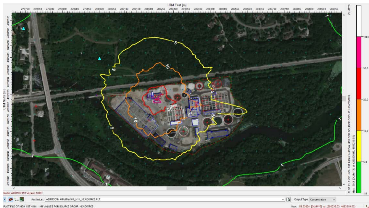
Figure 4-5. Maximum 1-hour Odor DT Raw Sewage Influent Lift Station and S&G Building
