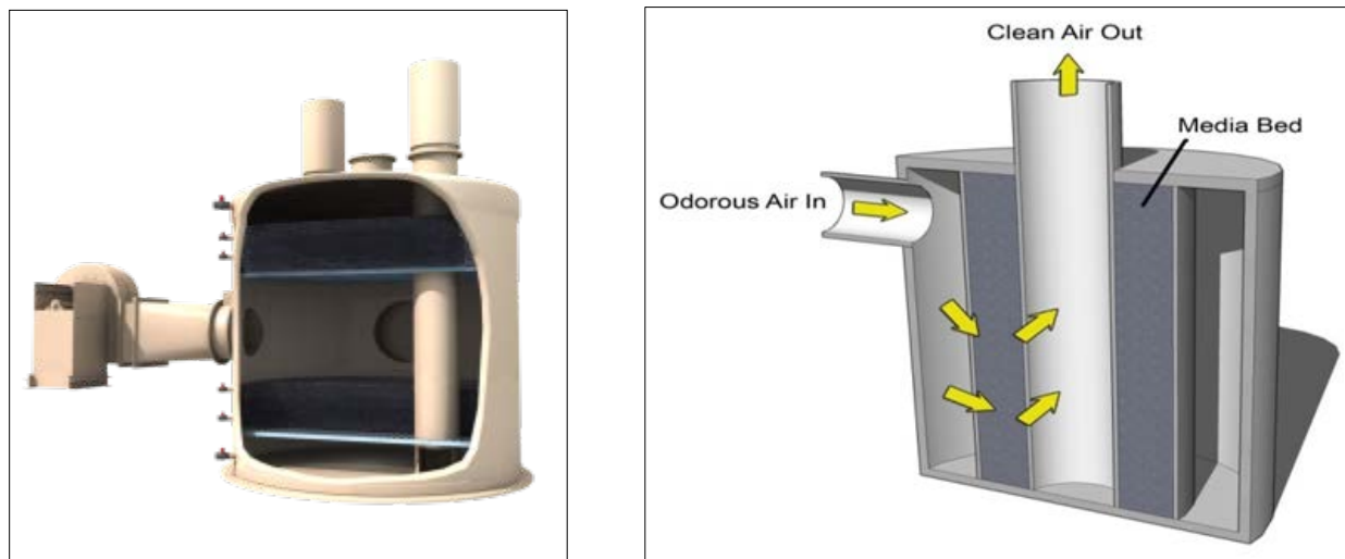
Figure 5-2. Schematic of Dual Bed (left) and Radial (right) Carbon Beds
