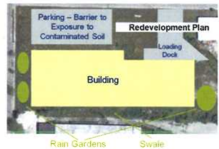
Example redevelopment plan using green infrastructure while placing barriers over contaminated soils.
