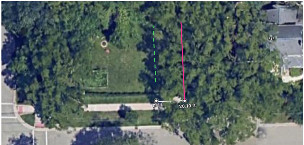
Figure 4 – 20-foot construction setback point from the proposed property line. Falls just outside of the Walnut canopy
