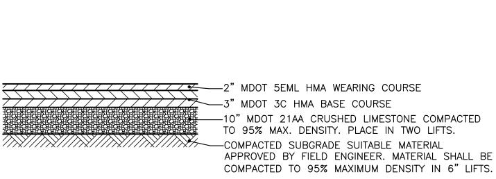
5.5" HMA ROADWAY PAVEMENT DETAIL NOT TO SCALE
