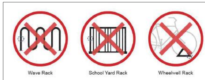
Figure 19-1. Prohibited Bicycle Parking Racks (source: 2024 AASHTO Guide for the Development of Bicycle Facilities)
