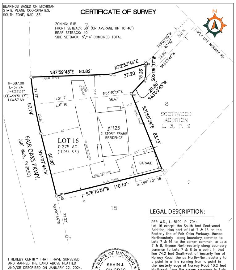
AND/OR DESCRIBED ON JANUARY 22, 2024, AND THAT THE RATIO OF CLOSURE ON THE UNADJUSTED FIELD OBSERVATIONS OF SUCH SURVEY WAS 1:5000, AND THAT ALL OF THE REQUIREMENTS OF P.A. 132, 1970, AS AMENDED, HAVE BEEN COMPLIED WITH.
