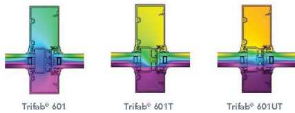
Thermal simulations showing temperature variations from exterior/cold side to interior/warm side.
