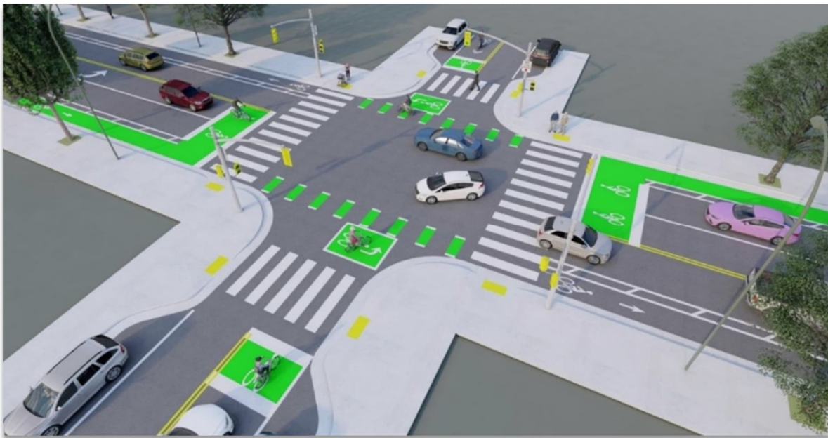
Figure 26 - Example of Bike lanes, Bike Boxes, and Conflict Markings at an Intersection 4
