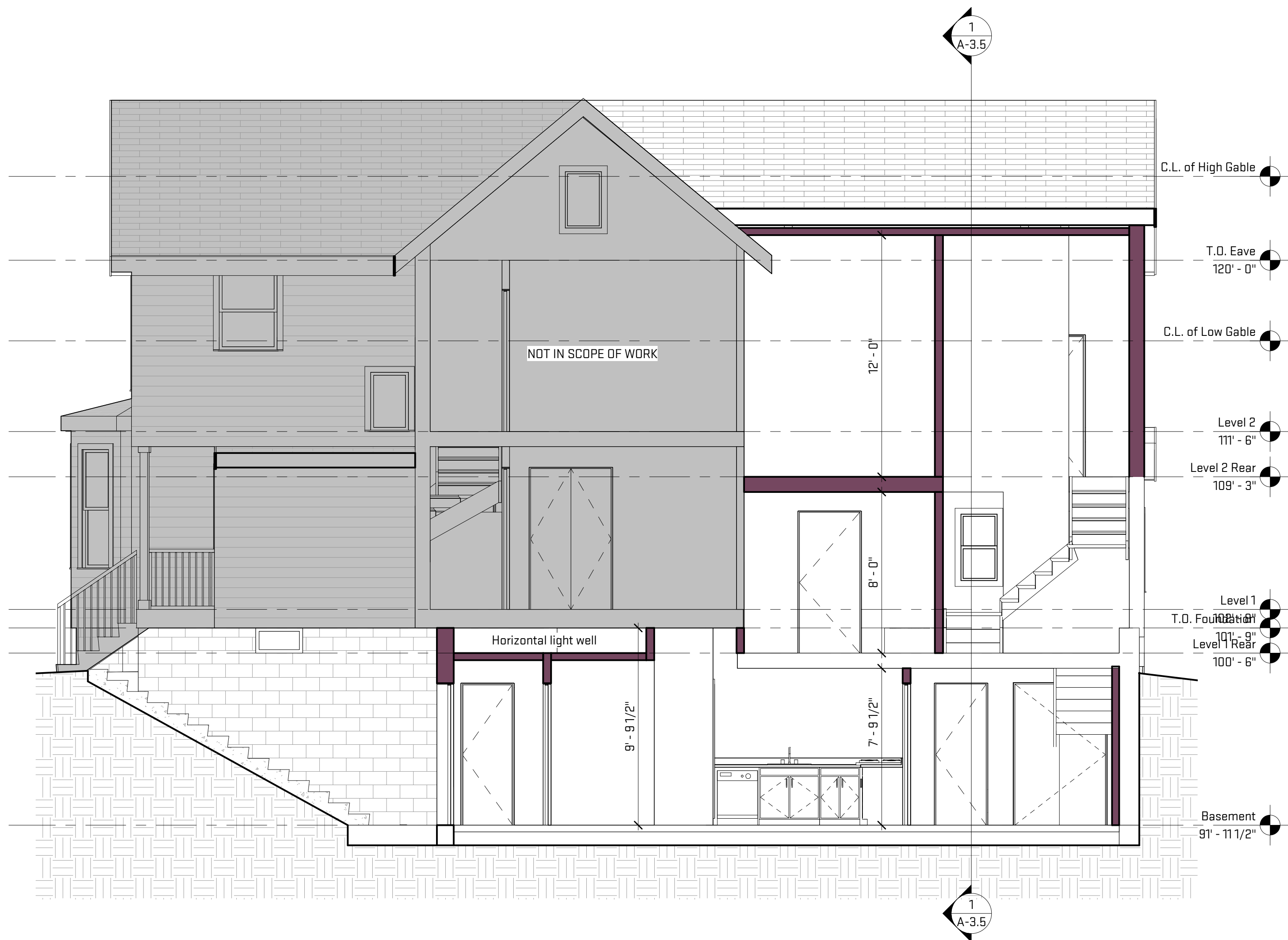
2 Long Section Through Basement Entry A-3.5 1/4" = 1'-0"
