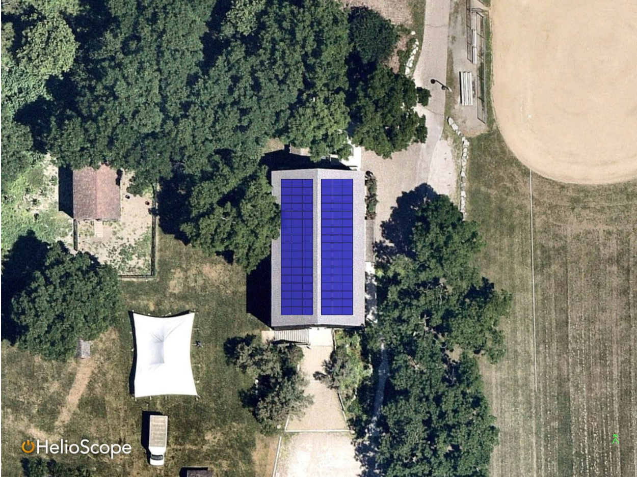
Layout 2 – 102 410W black panels, 41.82 kW DC, three rows in portrait
